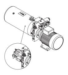
The W83AB series power pack is designed for applications that need high pressure and larger flow,but use a low-power B14 Frame motor. The power pack uses a special manifold (W800553). All screw-in cartridge valves have been designed to be adjusted easily to service the power pack quickly. They still have the same dimensions and functions as the standard manifold (W800532).
